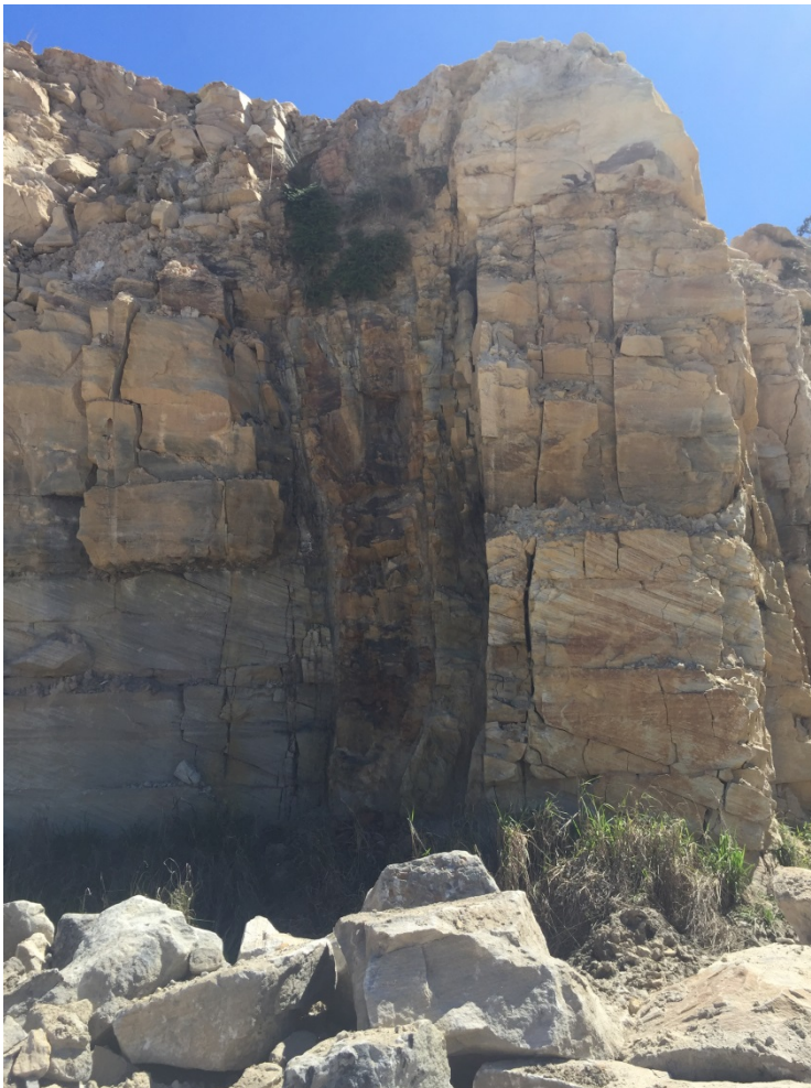
Photo 2: Weathered basaltic dyke in the northern wall of the quarry. The dyke is around 1 to 2 m wide and deeply weathered. No vertical displacement of the sandstone appears to have occurred across the dyke. Cross bedding within the sandstone beds is clearly visible.
