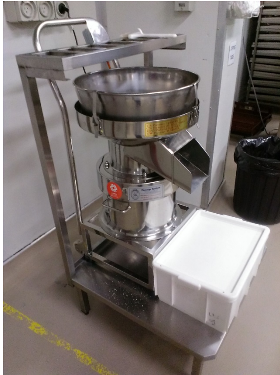
Figure A - 5: Sifter for cocoa and almond meal, showing internal extraction / filter
