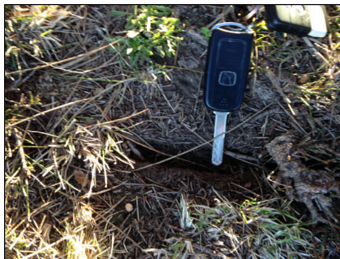
Figure 9 – Clay Surface Cracking
