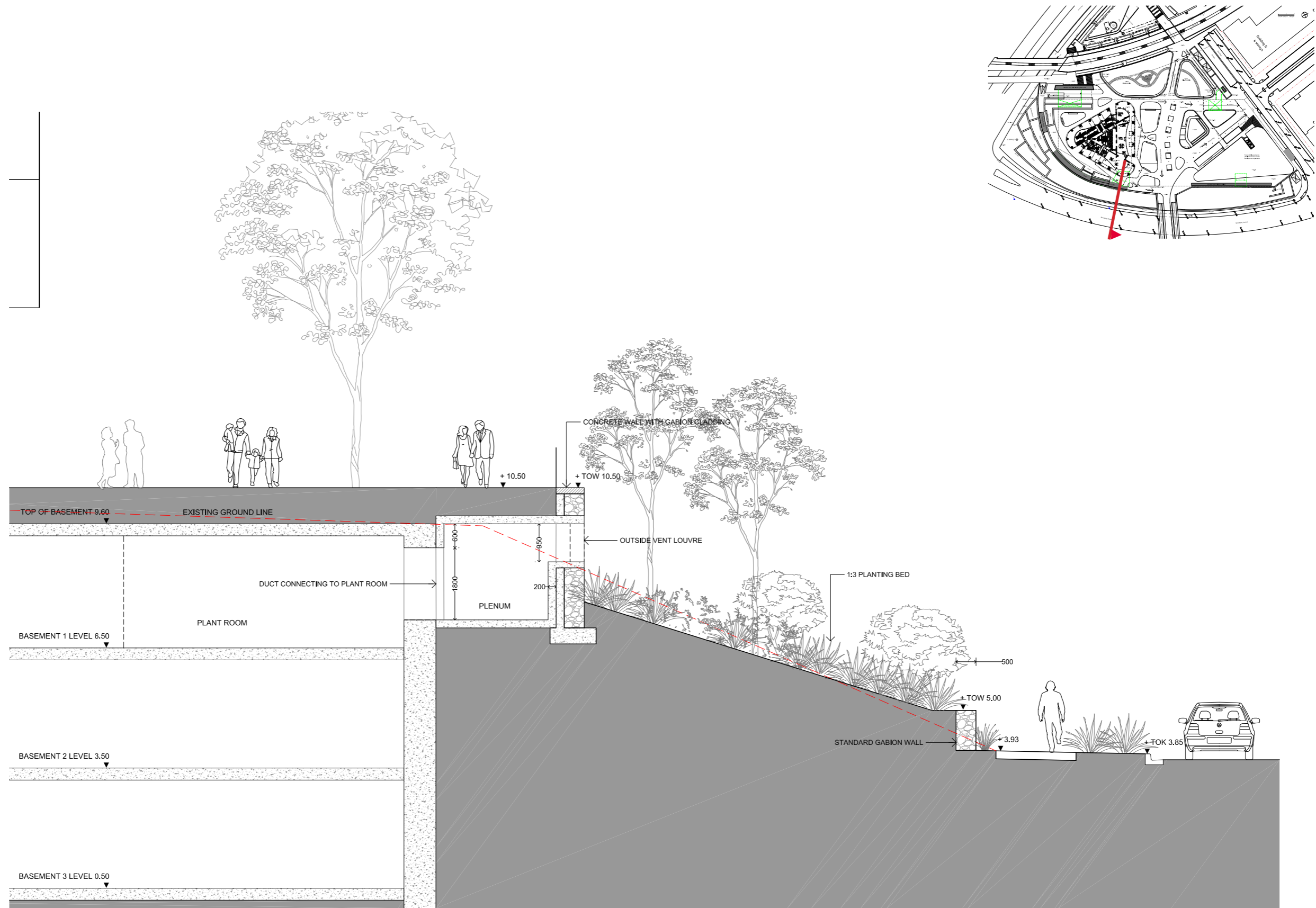
SECTION THROUGH EXHAUST VENT AND PLANTING BED
