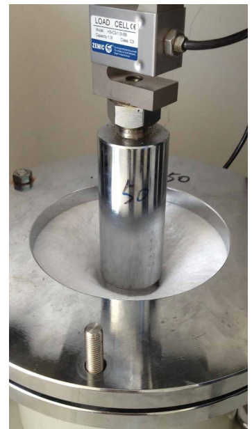
AS 3706.4 CBR BURST STRENGTH
