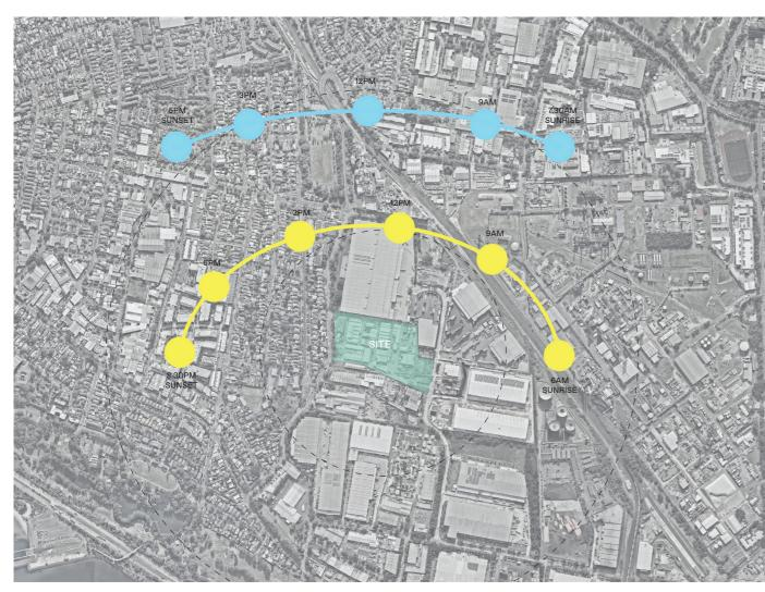
The east/west orientation of the warehouse buildings is a primary design consideration, providing excellent sunlight exposure for the installation of solar panels on the roofs. This orientation allows for efficient solar energy harvesting, supporting the building's sustainability goals.
