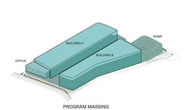
The building is divided into 3 massings, Building A, B & Office Block and a heavy vehicle ramp. Building A & B have a primary east/west orientation to maximise site efficiency. Heavy vehicle ramp structure is located on the eastern side and Office Block is sited along the western boundary.
