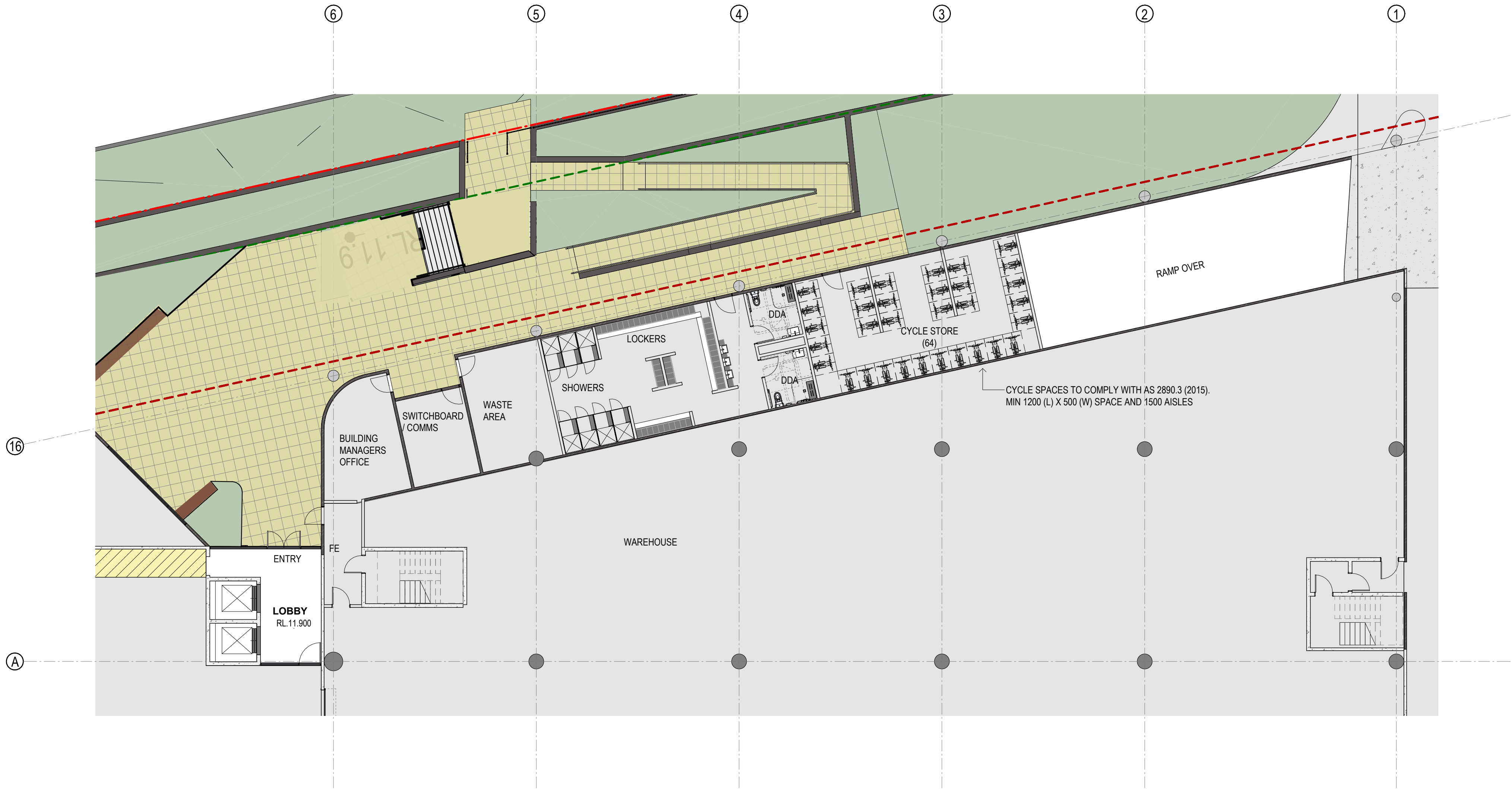
1 GROUND FLOOR - END OF TRIP FACILITIES 1 : 150
