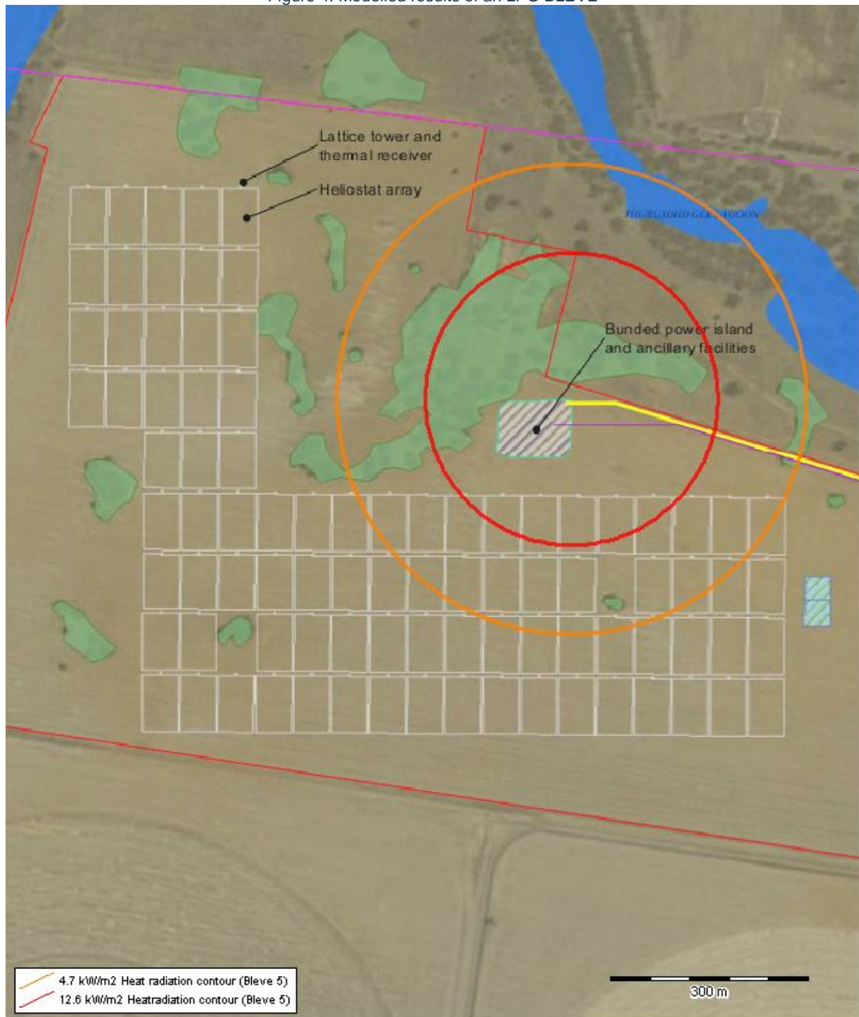
Figure 4: Modelled results of an LPG BLEVE
