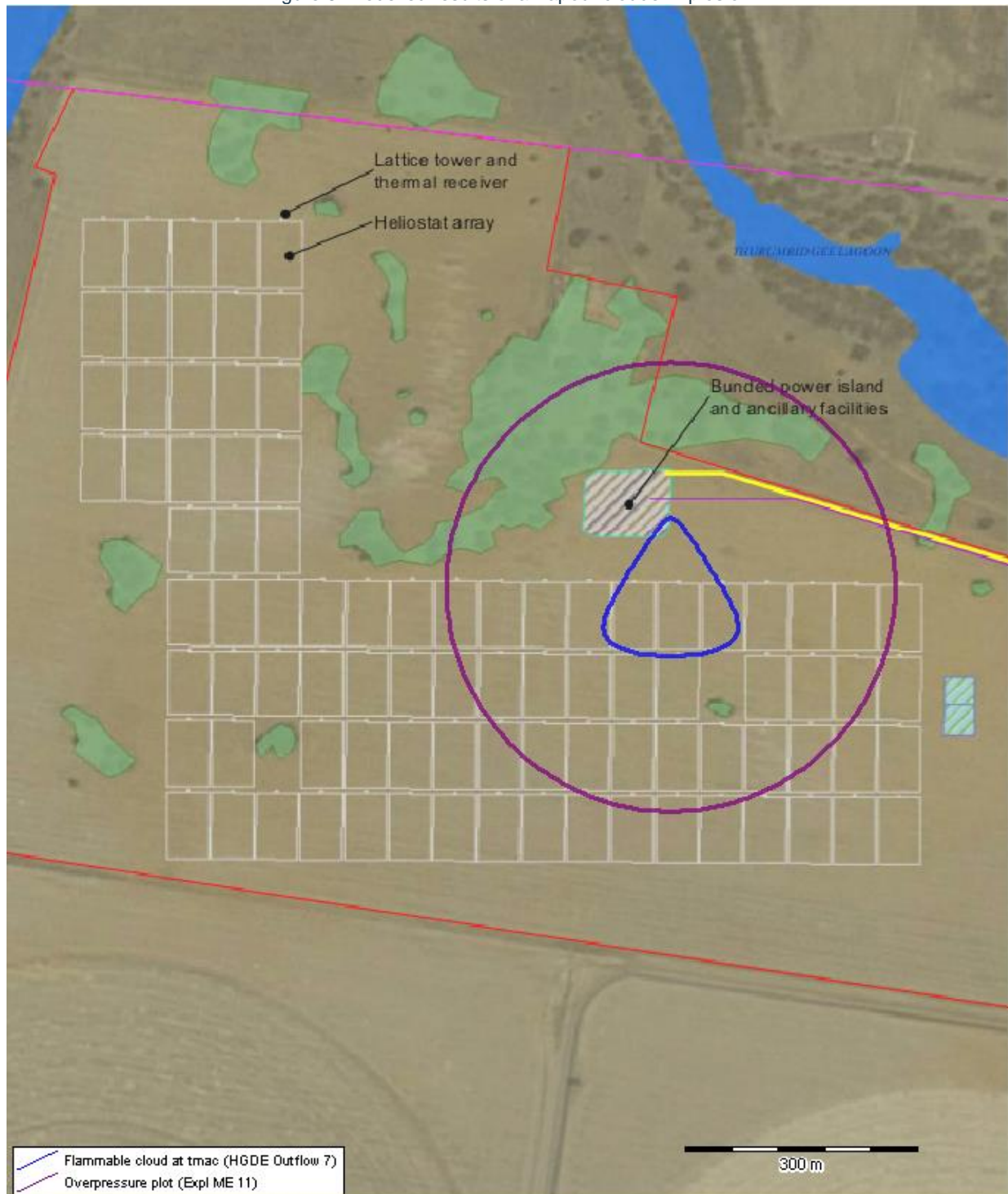
Figure 6: Modelled results of a Vapour cloud Explosion
