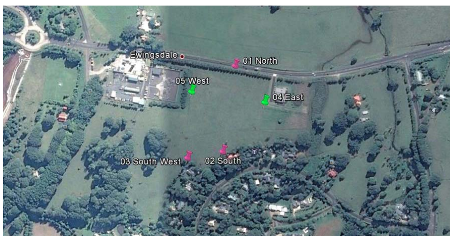
Figure 2 Location map of unattended noise logging (pink markers only) and operator attended measurements (pink and green markers)
