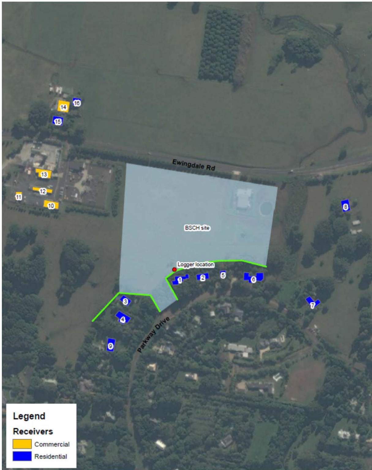
Figure 3 Construction noise modelling map
