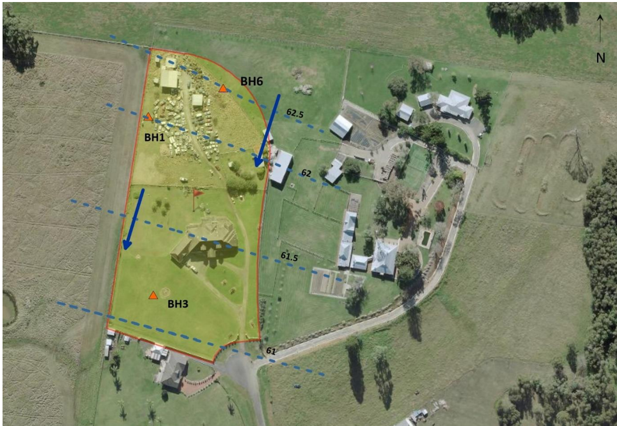
Figure 4 Interpreted groundwater flow direction (28 th February 2024) -dashed line represent interpreted piezometric level (mAHD) and arrows interpreted flow direction
