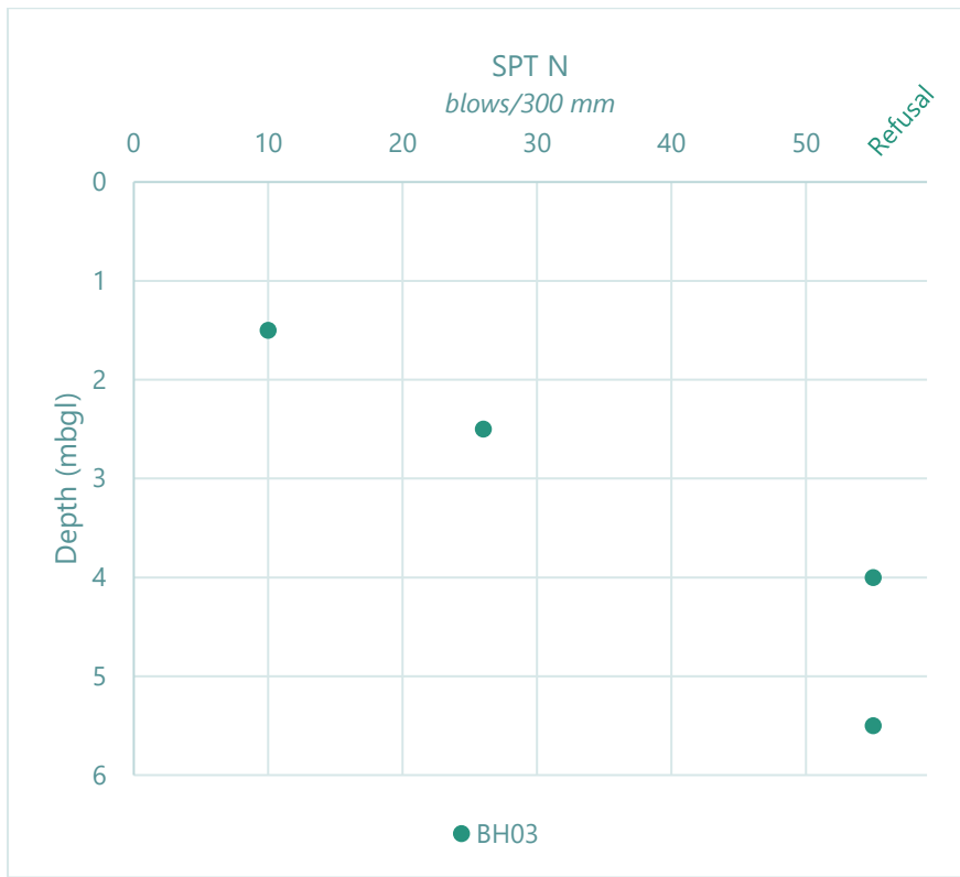
Figure 3-4: SPT N – depth profile plot
