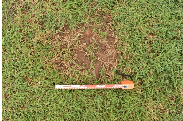
Figure 20: Orange brown clay visible in areas of ground exposure indicating the removal of natural topsoils
