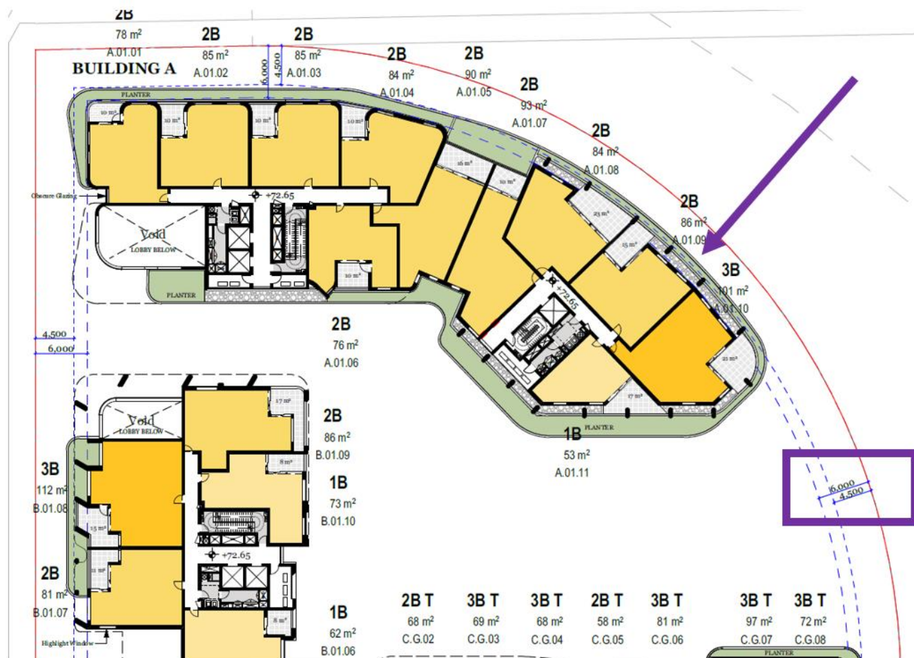
Figure 42 Example of setback exceedance (beyond 4.5m) at Building A
