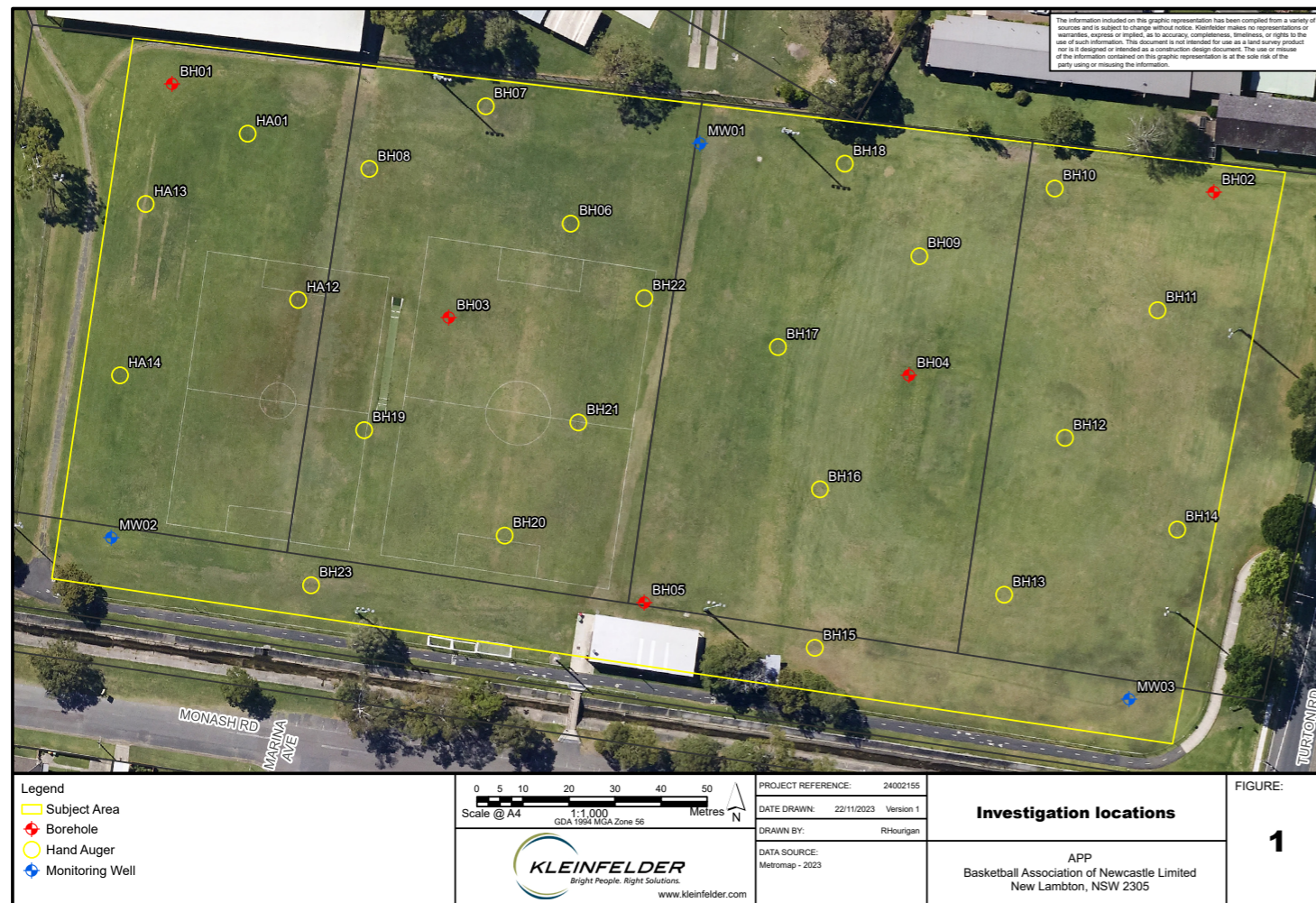
Figure 9: Geotech Bore Hole Locations
