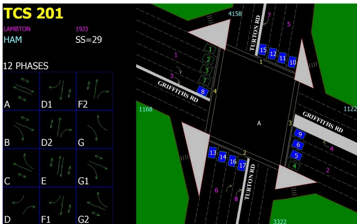
Figure 3.3: Turton Road / Griffiths Road - TCS 201 Signal Phasing
