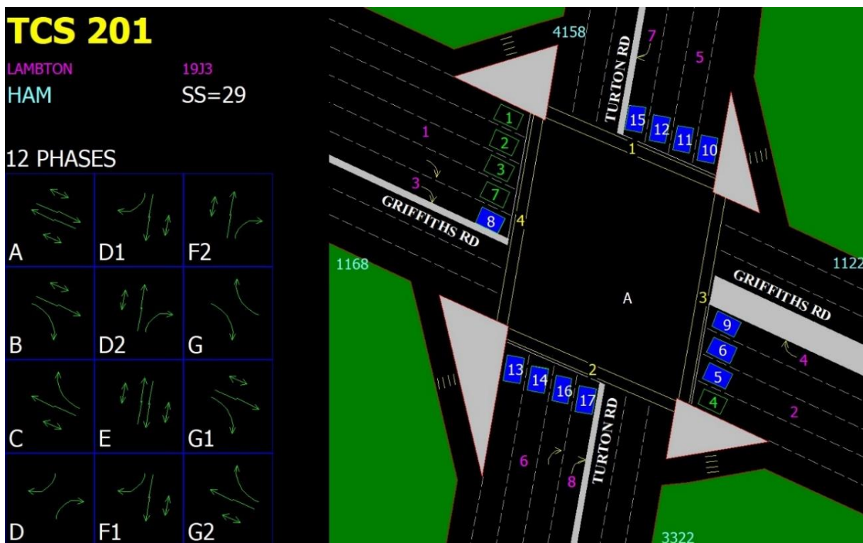
Figure 3.3: Turton Road / Griffiths Road - TCS 201 Signal Phasing
