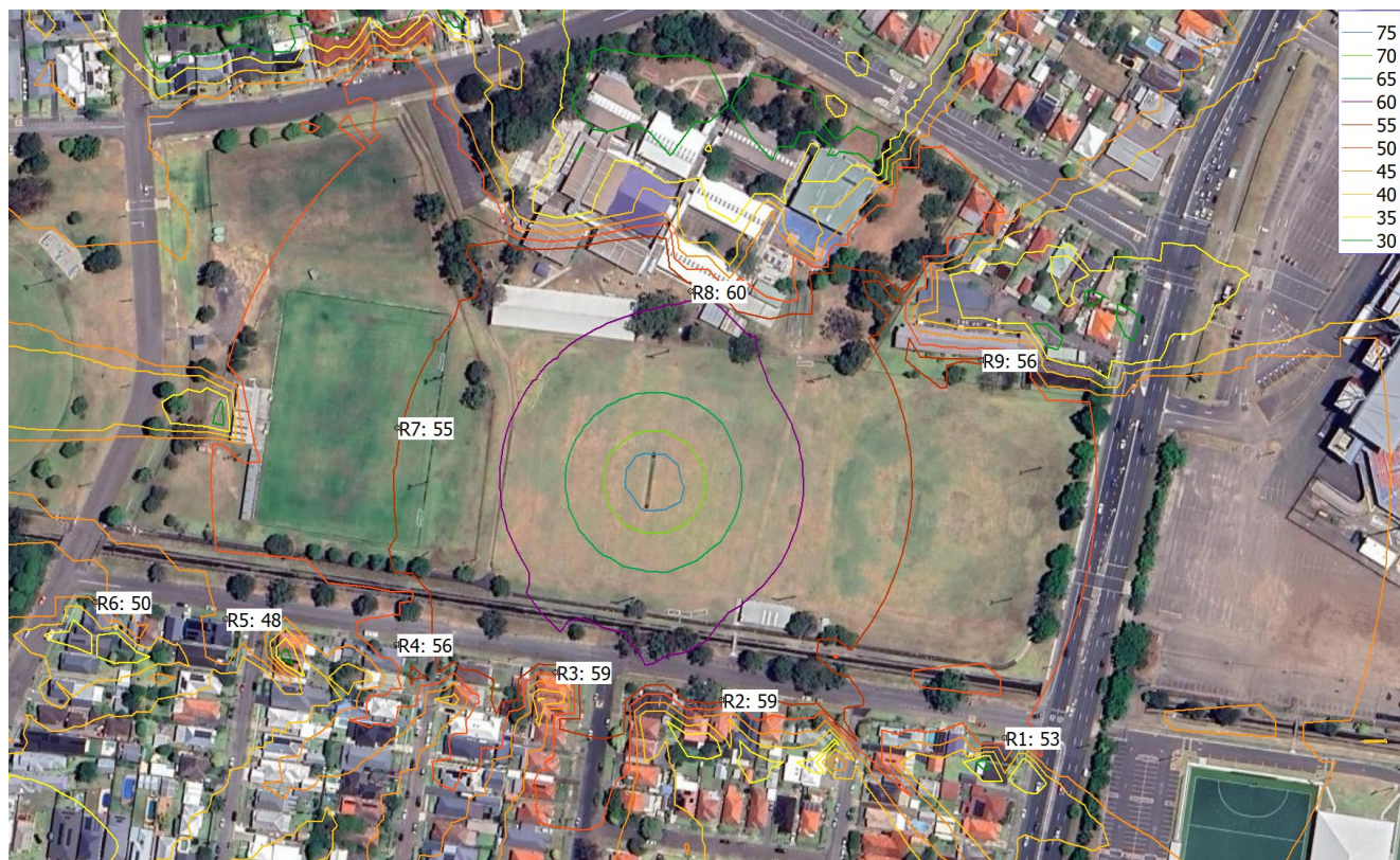
Figure 4-4 Construction Excavation West dB(A) Leq(15min)
