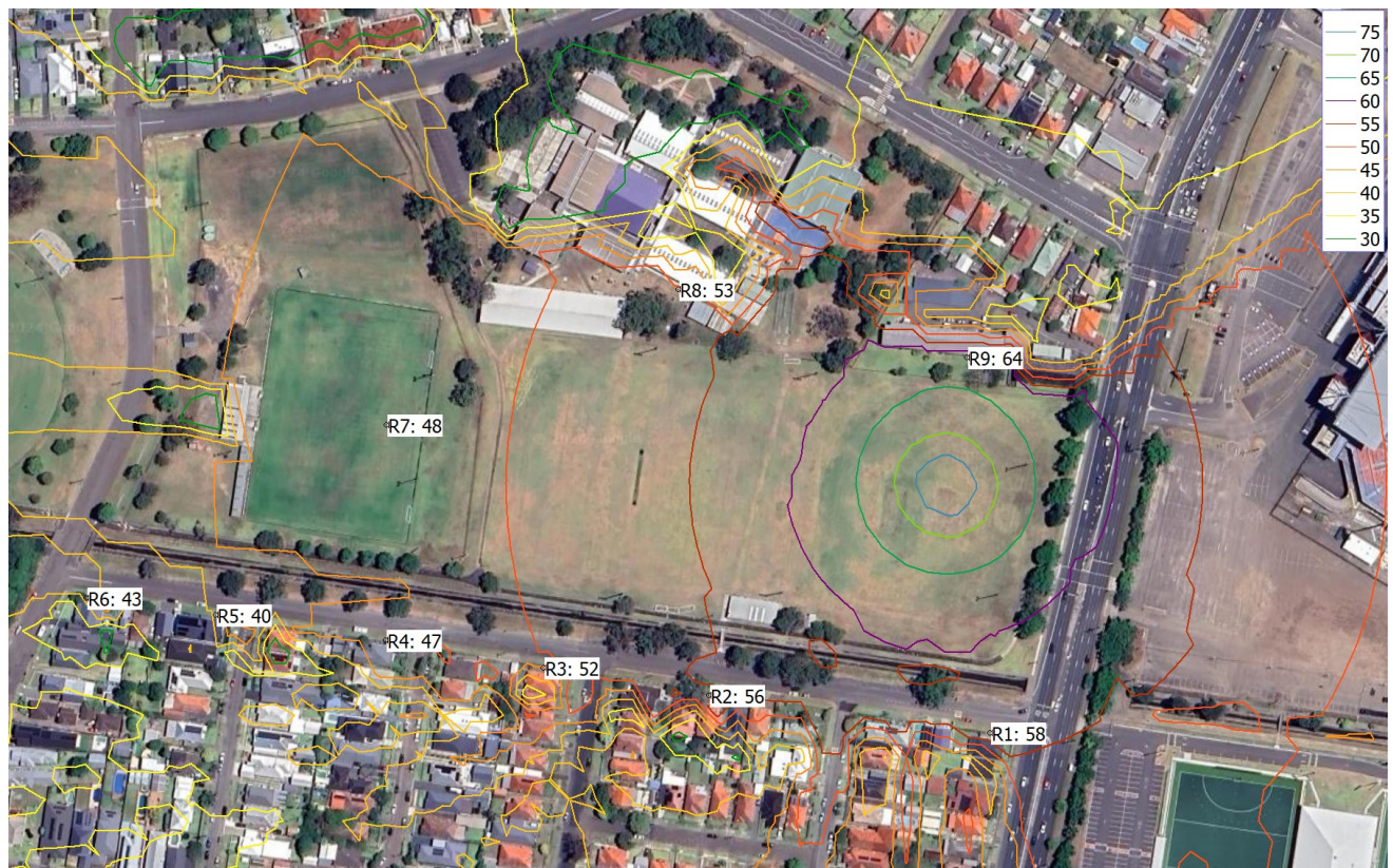
Figure 4-2 Construction Excavation East dB(A) Leq(15min)
