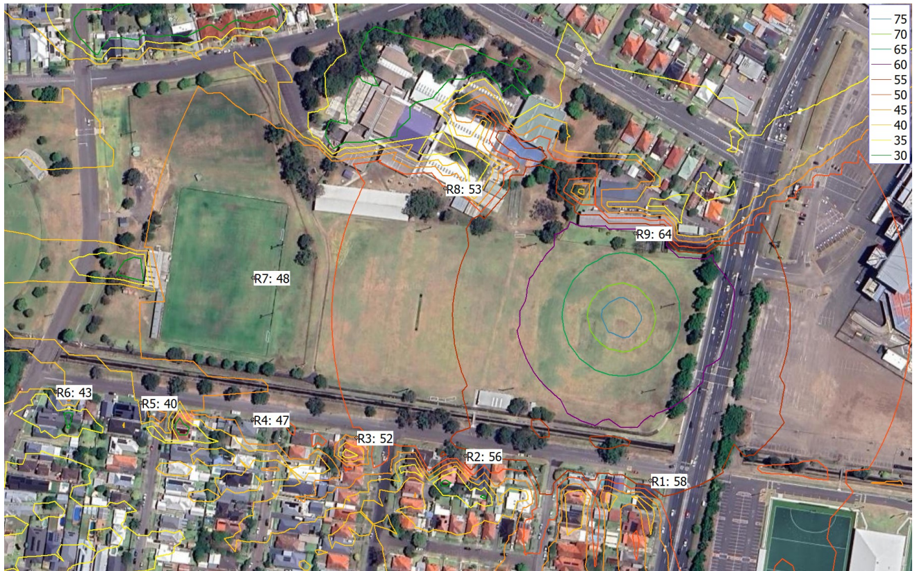
Figure 4-2 Construction Excavation East dB(A) Leq(15min)
