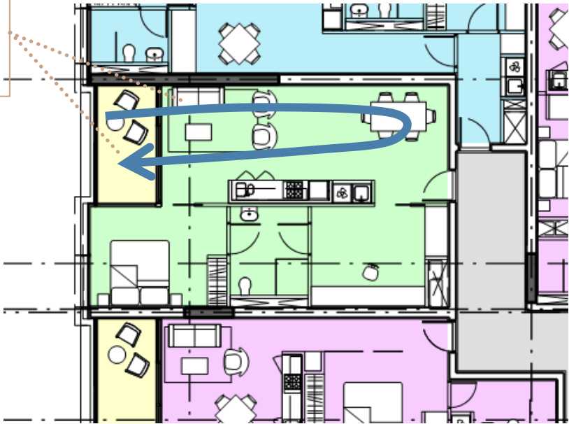
Figure 9: Natural cross ventilation paths through the selected apartment
