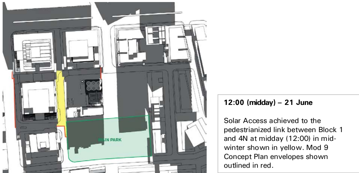
Figure 3 – Additional solar access from Block 1 +4N envelope – compared to previous approved scheme.
