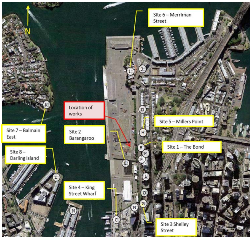
Figure 7: Surrounding receivers identified (A to P) & Noise logging locations (1 to 8)
