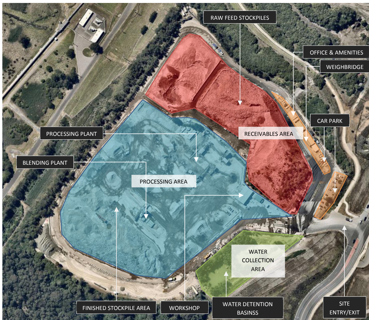
Figure 3 Site layout of the Widemere Recycling Facility
