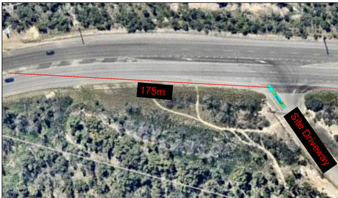
FIGURE 4: DRIVEWAY SIGHT DISTANCE - SOUTH
