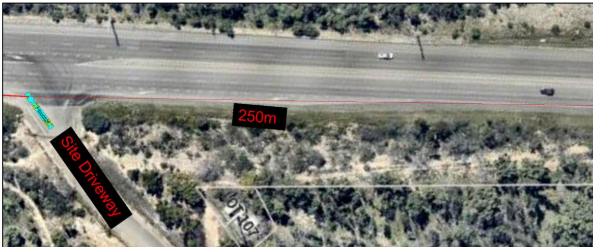
FIGURE 5: DRIVEWAY SIGHT DISTANCE - NORTH
