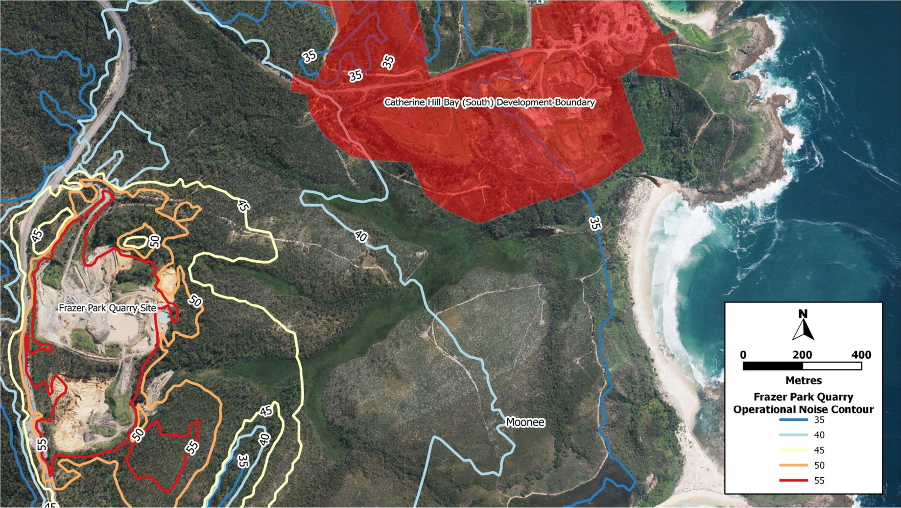
Figure 6-1 Typical Worst-Case Operational Noise Contour – L_{Aeq,15min} (dBA)
