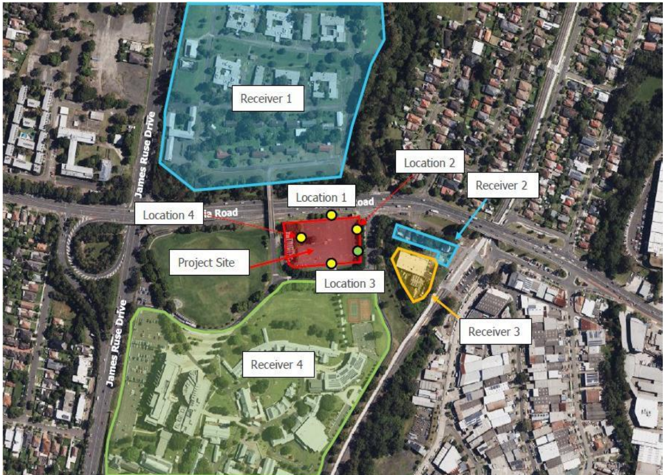
Figure 4 Site Map, Nearest Sensitive Receivers, Monitoring Locations. Source: Pulse White Noise Acoustics.
