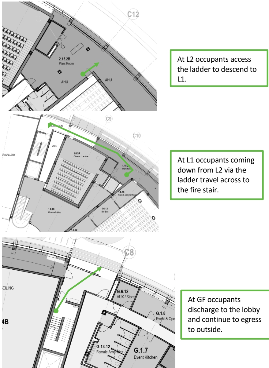
Figure 14.1: Discontinued egress path from L2 to outside at GF
