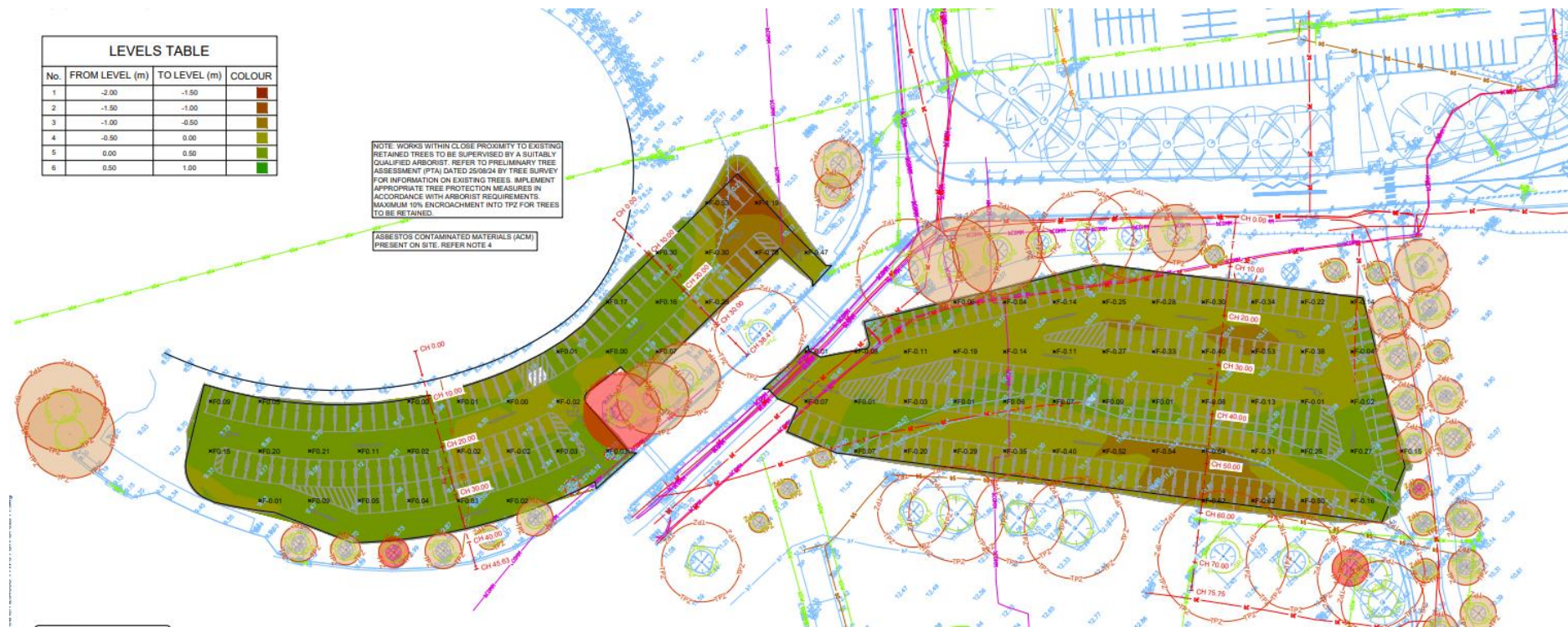
Figure 6-4: Bulk Earthworks Cut and Fill Estimates. Source: TTW 2025.
