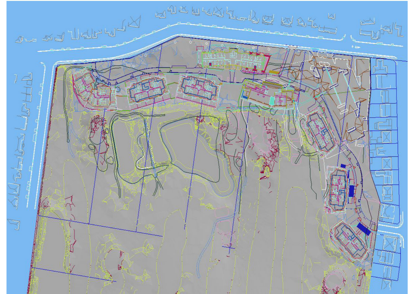
Image showing survey drawing from Crux Surveying at MGA 56 GDA2020 coordinates aligned to 3D model (grey)
