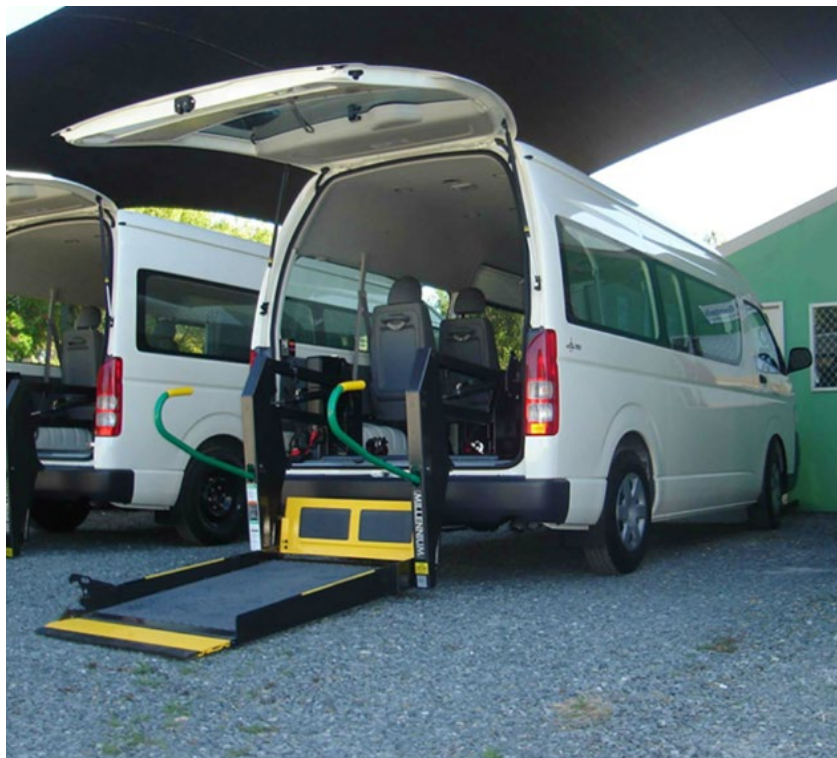
Figure 4: Indicative Village Bus providing for accessible travel
