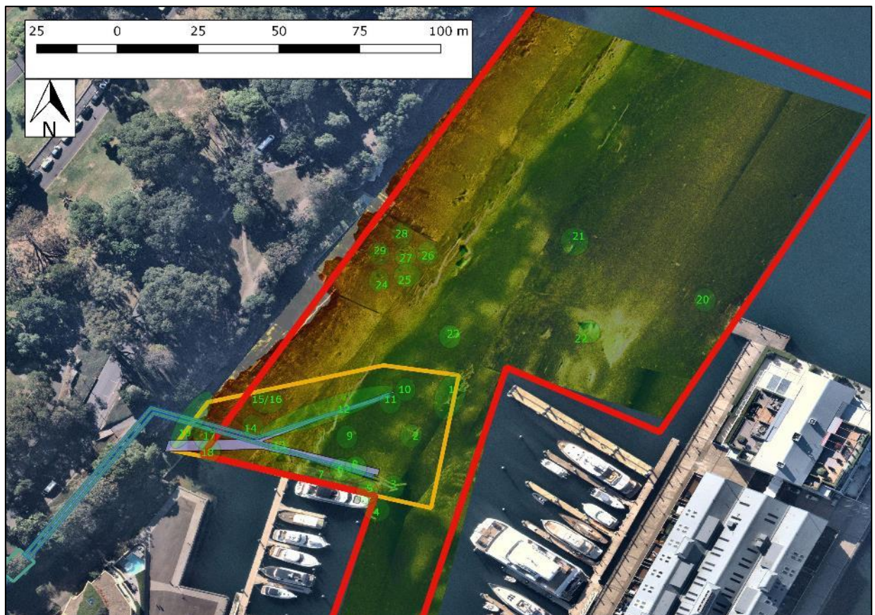
Figure 7: Overlay of MBES and SSS imagery with distribution of targets identified for dive inspection
