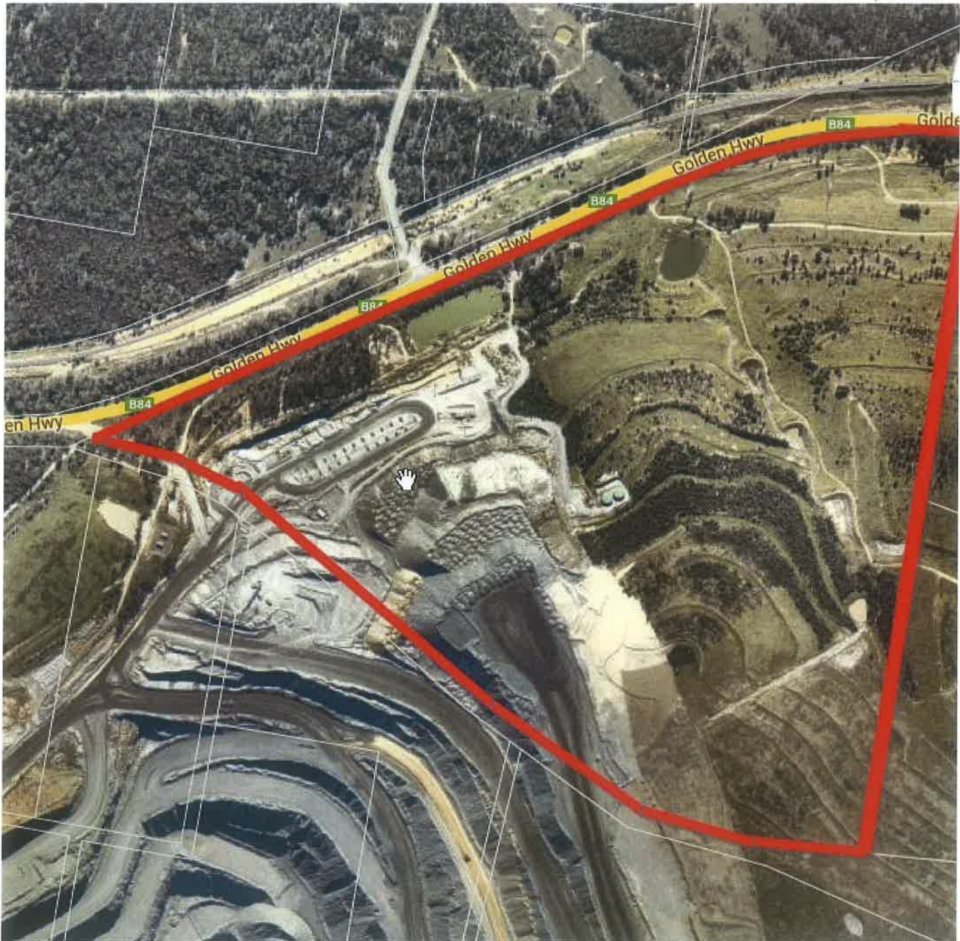
Diagram 1: Lot 2011 DP 1137289 shown with red border. The impacts and extent of open cut mining disturbance requiring landforming and rehabilitation is shown. Source of imagery – Nearmaps; Date of imagery 1 July 2014.
