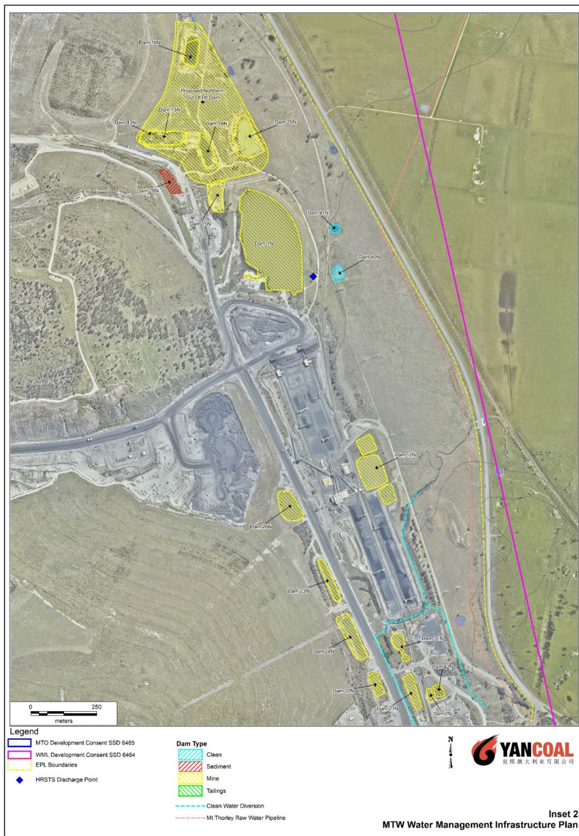
FIGURE 24B – MTW WATER MANAGEMENT INFRASTRUCTURE PLAN - INSET 2 (WML DETAIL)
