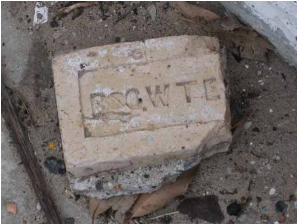
Figure 53. Semi-plastic brick on Gibson Street site, bearing frog of Joseph Bowtell. EJE
