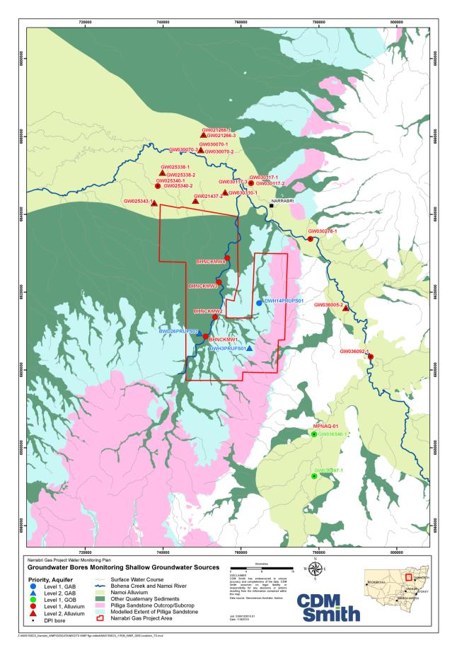
Figure 3-9 Groundwater bores monitoring shallow groundwater sources
