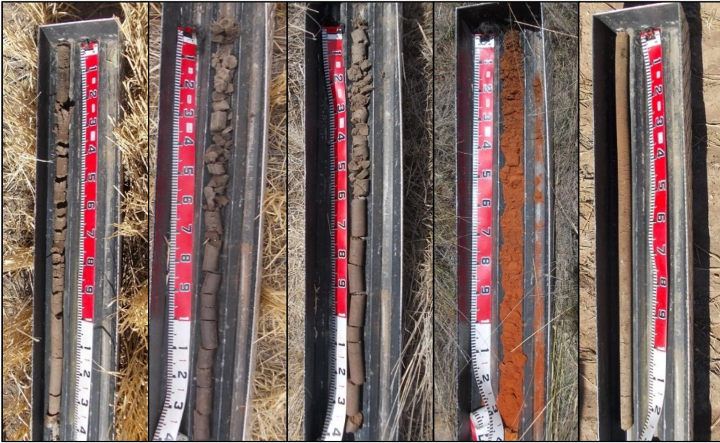
Figure 6 Soil profile cores from each representative unit: (L to R) slight gilgai Vertosol; medium gilgai Vertosol; strongly gilgai Vertosol, Sodosol, Red Kandosol
