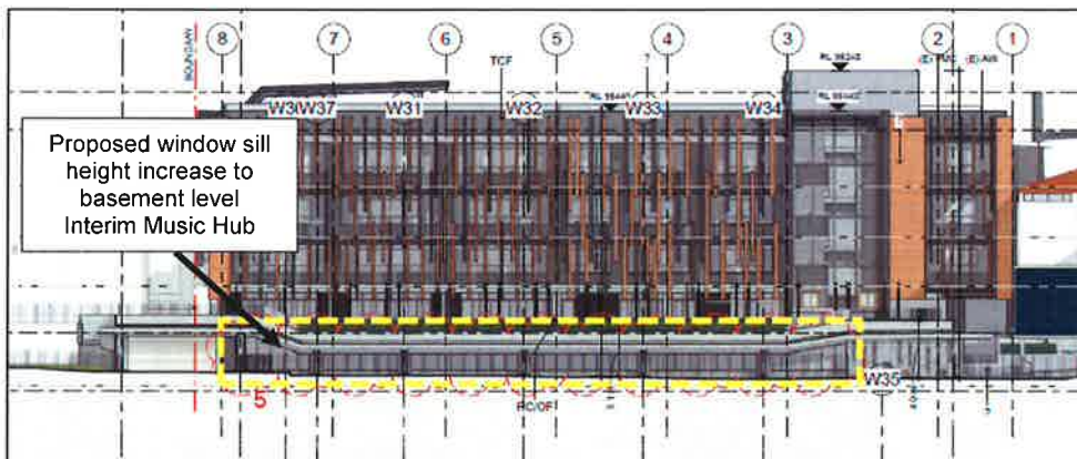
Figure 8: Extent of area affected by increase in sill height (shown dashed in yellow, Source: Submitted Modification 1 plans)
