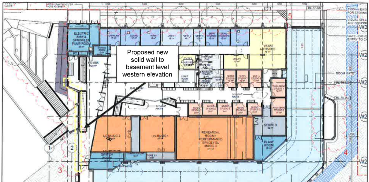
Figure 7: Area of foyer glazing to be replaced by solid wall (shown dashed in yellow, Source: Submitted Modification 1 plans)
