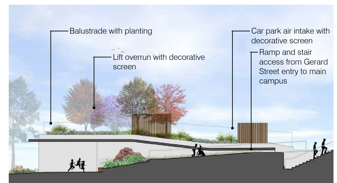
SECTIONAL ELEVATION THROUGH MAIN ENTRY
