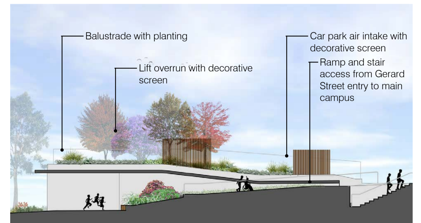
SECTIONAL ELEVATION THROUGH MAIN ENTRY
