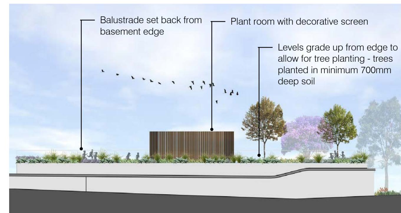
SECTIONAL ELEVATION THROUGH EASTERN BASEMENT WALL
