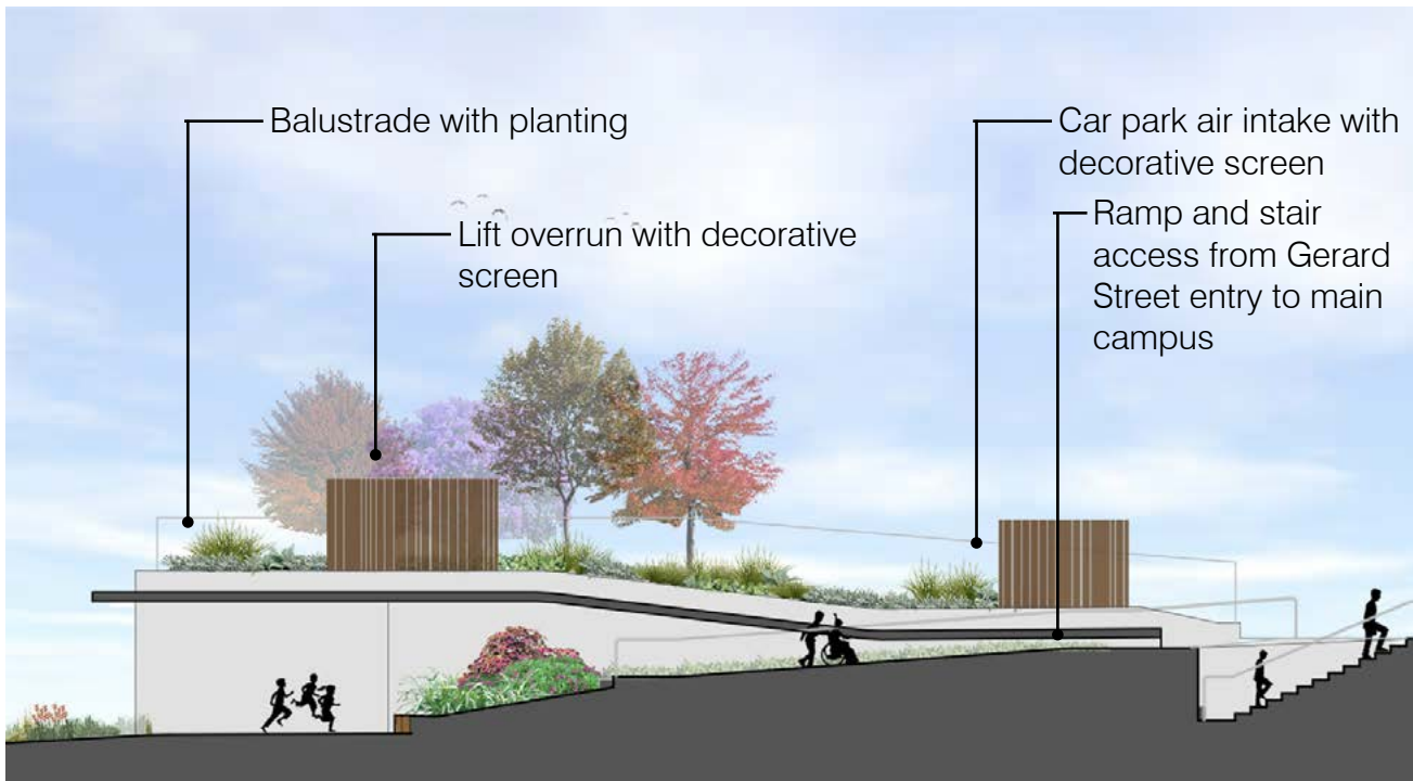
SECTIONAL ELEVATION THROUGH MAIN ENTRY
