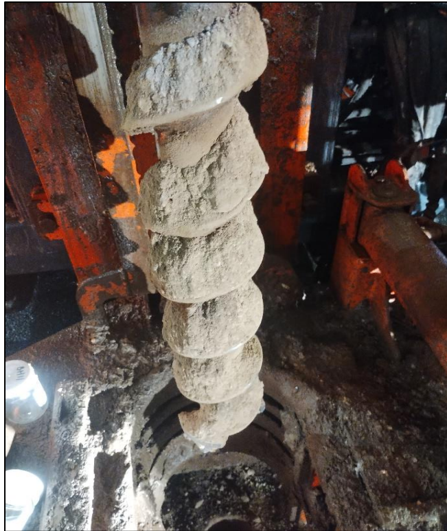
Photograph 27 - Shale encountered at BH11.
