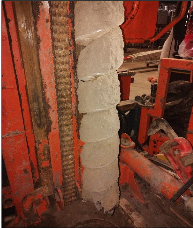
Photograph 15 - Gravelly clay fill material observed at BH2A.
