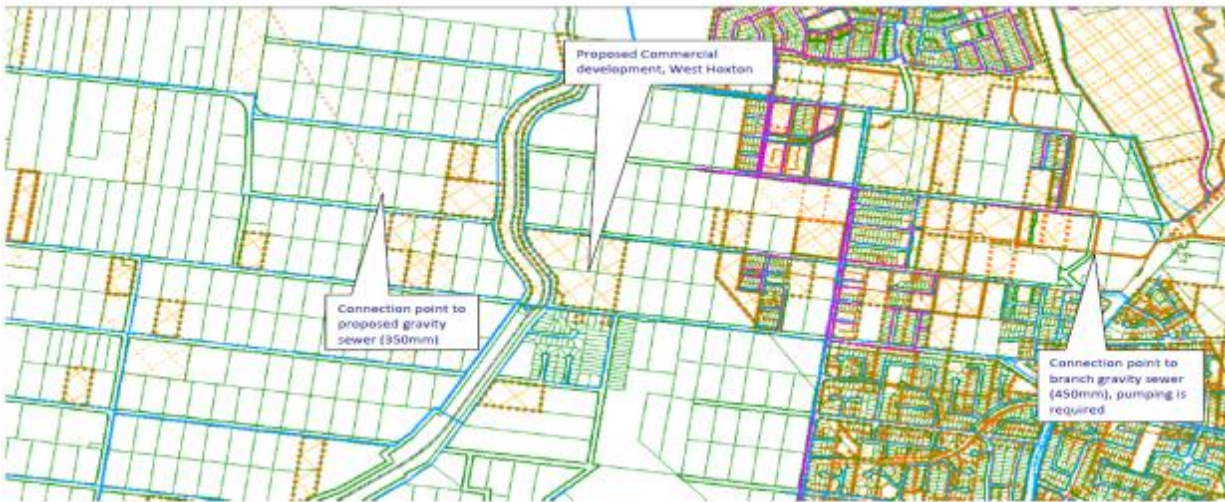
Figure 2 – Development location and sewer connection point
