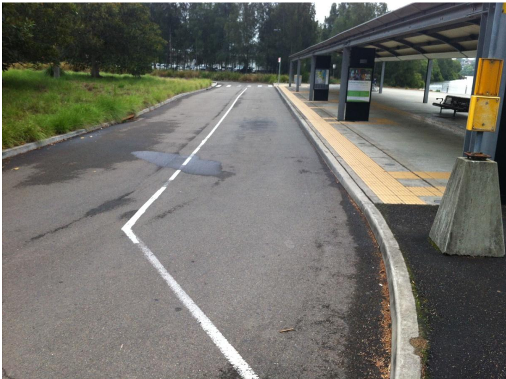
Figure 5: STA Bus Zone for up to 4 buses, bike rack for 26 bikes, zebra crossing
