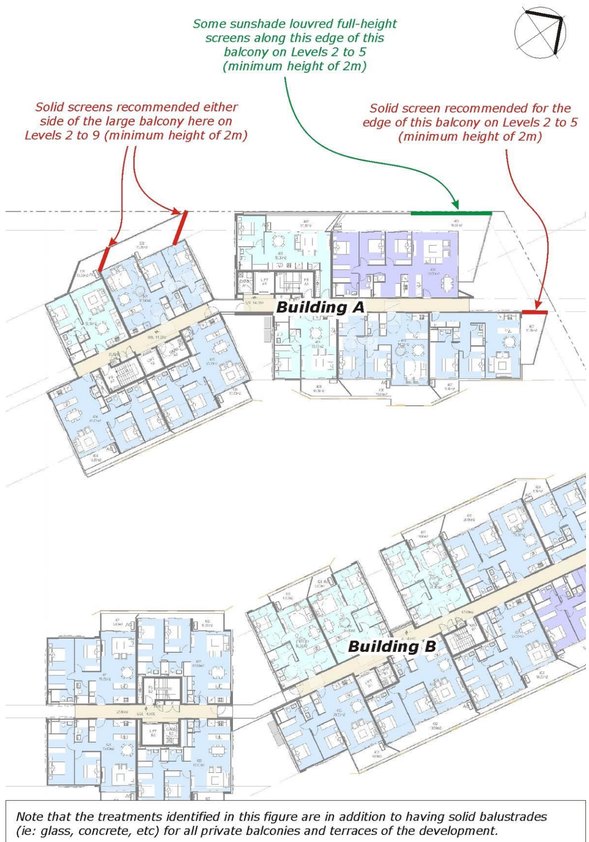
Figure 4c: Recommended Treatments for the Private Balconies and Terraces of Building A (Level 4 plan shown)
