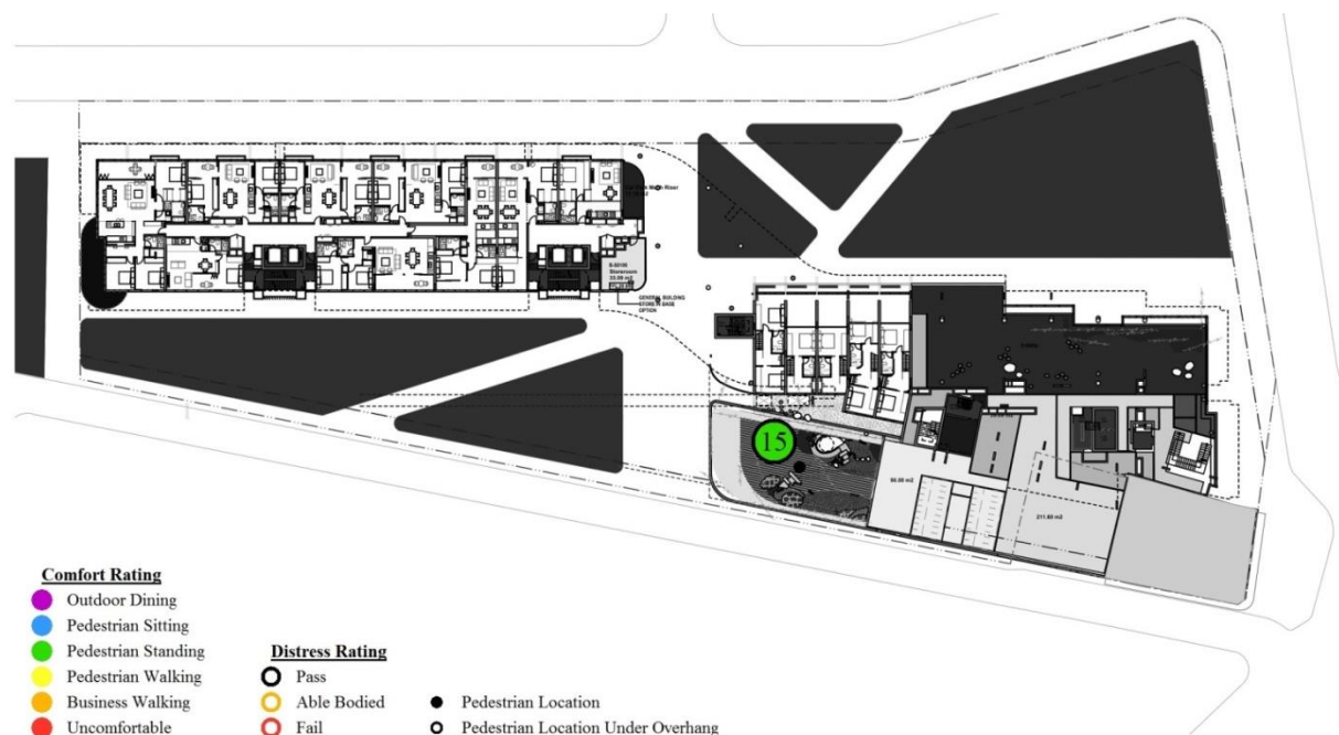
Figure 7: Pedestrian wind speed measurements locations at Level 1
