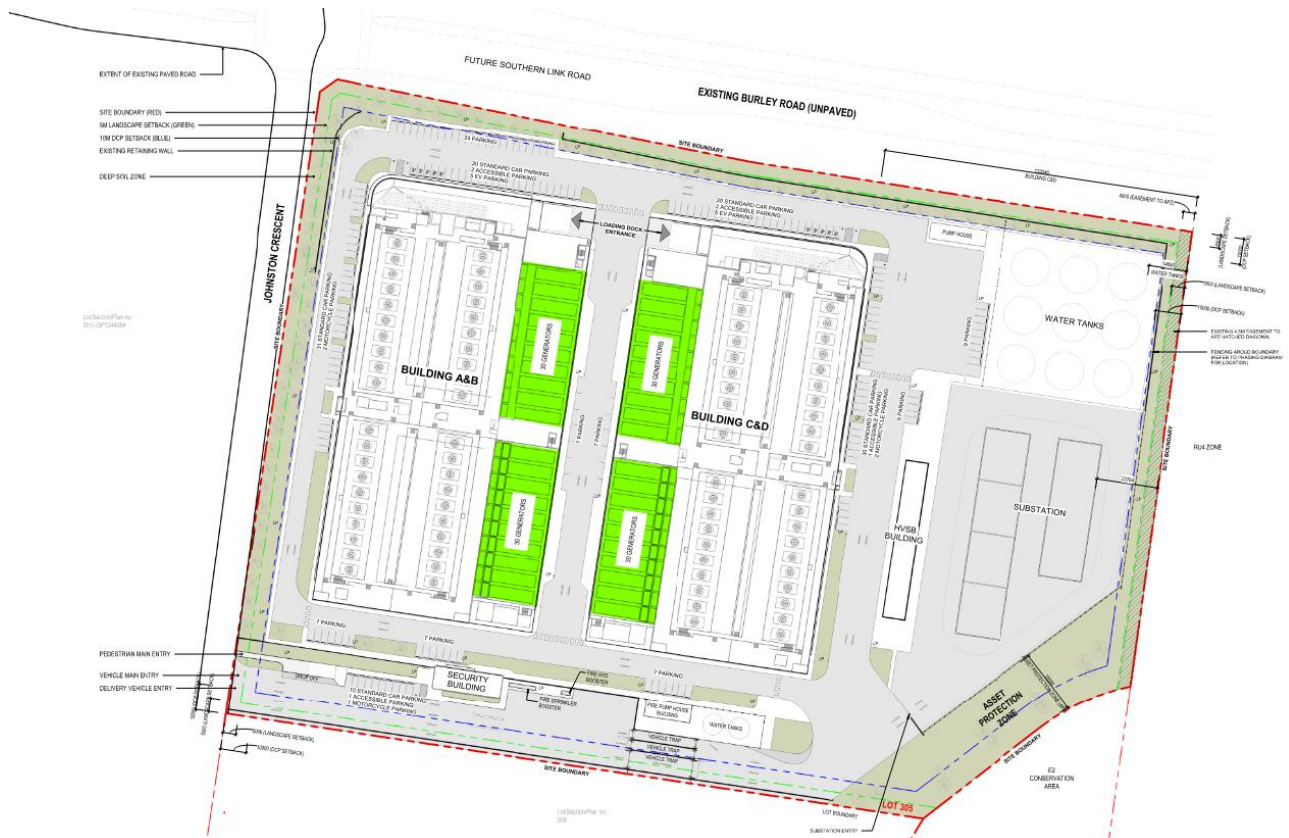
Figure 5.1.1 Location of Generators on Proposed Site (Green)
