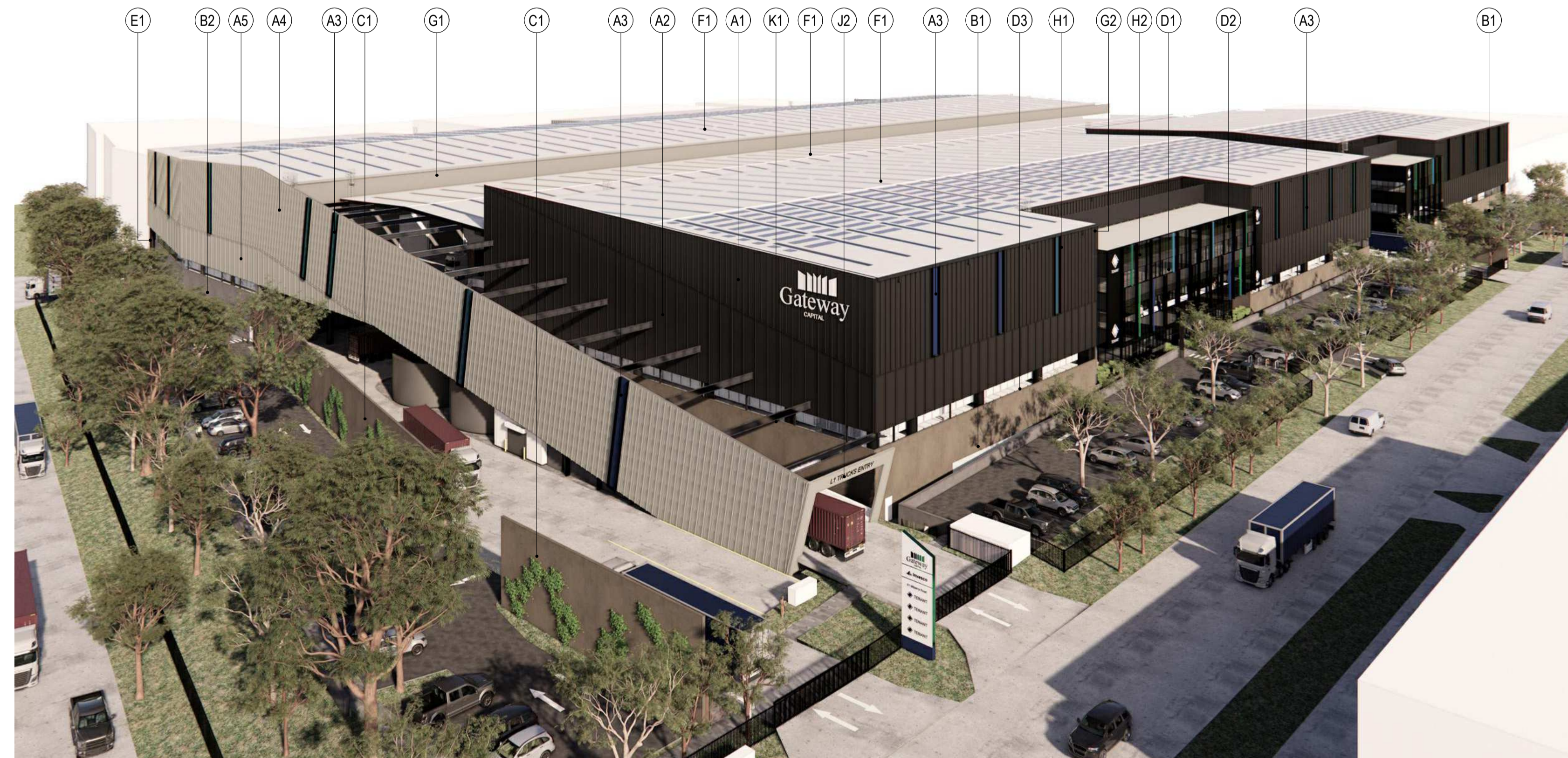
H1 ALUMINIUM WINDOW SHROUD TO WAREHOUSE EXTERNAL WALL (APPROX 6-10mm THICK x 300-400mm DEEP) BLACK
