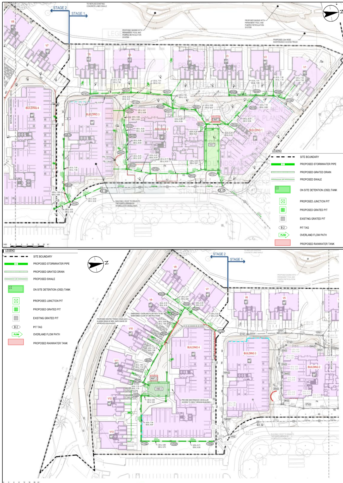
Figure 7-5: Stormwater Drainage Plan showing proposed rainwater tanks, on-site detention basins, pipes, and pits within the Stage 1 and Stage 2 bounds (Stantec, 2024b)
