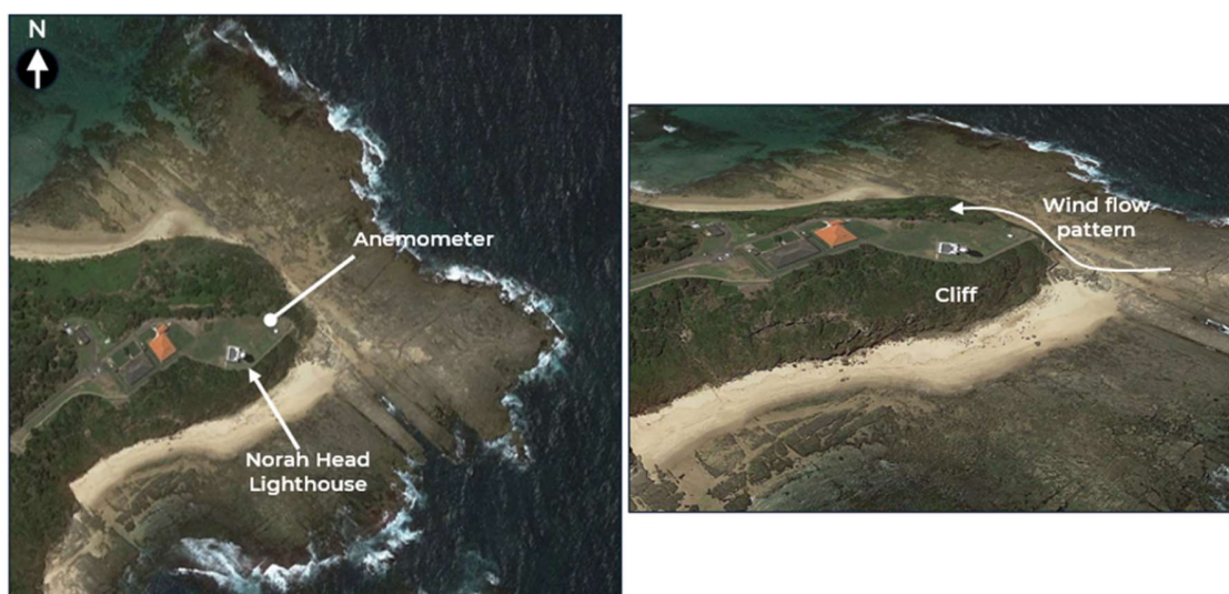
Figure 21: Overhead view showing location of wind data extraction site and anemometer.
