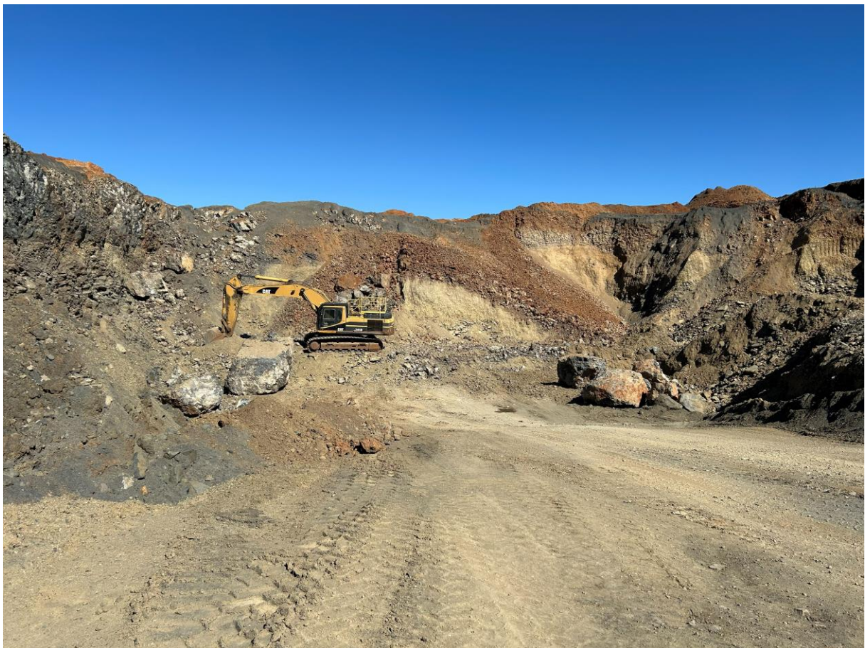
Photo 14: Excavator moving overburden in the western part of the pit.
