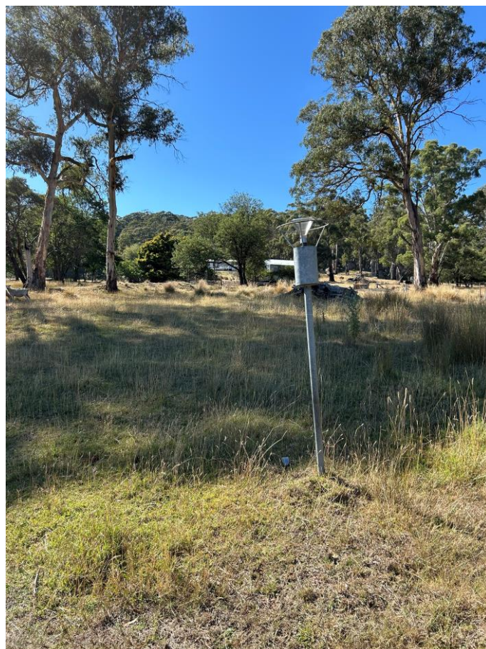
Photo 4: Deposited dust gauge on southern side of access road on adjoining lot.
