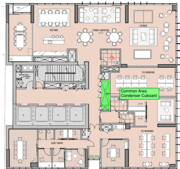
Common Areas Condenser Cupboard
