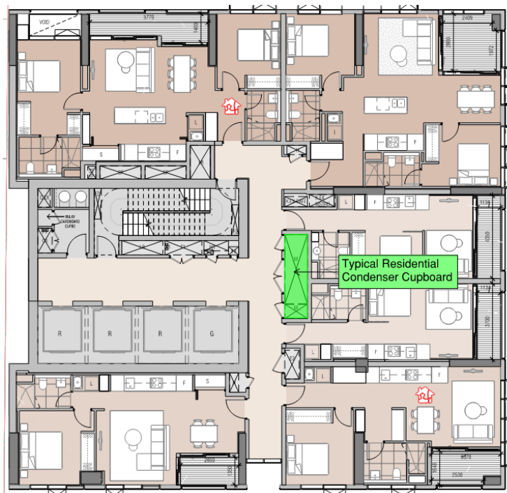
Typical Floor by Floor Condenser Cupboard
