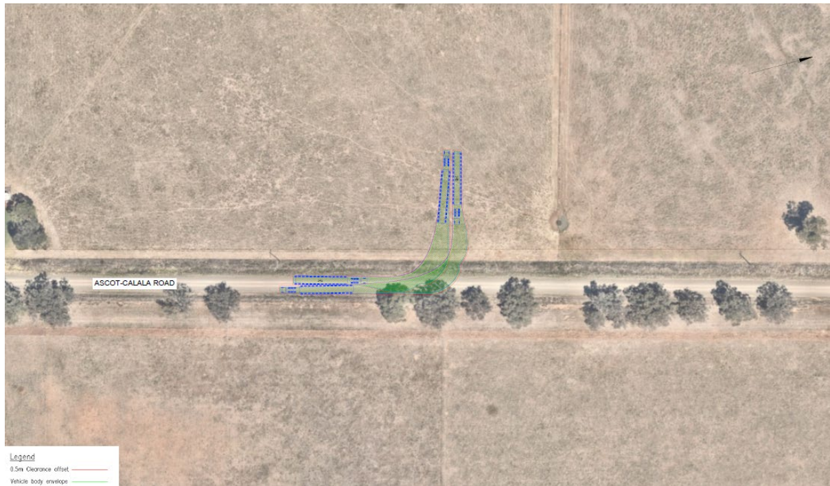
Figure 4-6: Ingress and egress of 35-metre long OSOM vehicle to and from the Project
